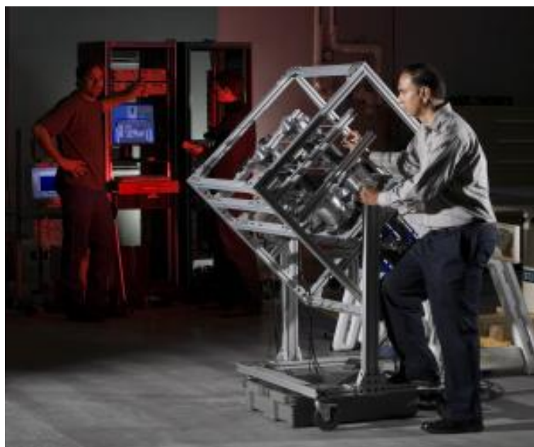
Nick Mascarenhas, physicist and principal investigator, prepares the detector for a test. The neutron scatter camera detects radiation at significant standoff distances and through shielding, and pinpoints radiation sources. (Credit: Photo by Randy Wong)
